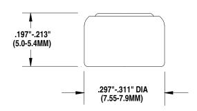
DIMENSIONS SHOWN ARE ANSI/IEC STANDARDS. FOR ENGINEERING TOLERANCES CONTACT RAYOVAC.
